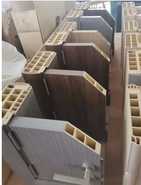
Figure A3 - Supplier factory reference: leaf/frame assembly and hollow profile geometry.
